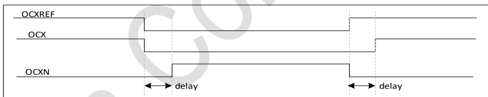
Figure 19-35 Complementary output with dead-time insertion
